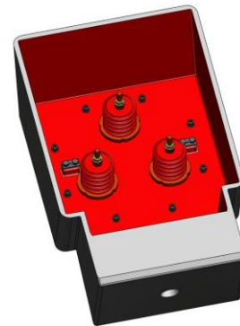
Figure 8-14 – Inside view of PTB
